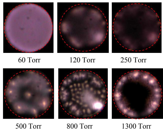
Figure 3: Exemplary visible photographs of CBLD operated in krypton at pressures from 60 to 1300 Torr. Pattern formation can be clearly seen from pressures of 120 Torr and beyond.
