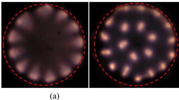
Figure 4: Self-organized pattern formation in krypton at 250 Torr at discharge current of (a) 0.647 mA and (b) 0.535 mA.
