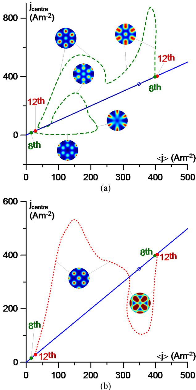
Figure 2: Bifurcation diagrams, Kr, 100 Torr,  $R = h = 0.5$  mm. Solid: fundamental mode. Dashed: 8<sup>th</sup> 3D mode. Dotted: 12<sup>th</sup> 3D mode. Full circles: bifurcation points. Open circles: point of minimum of the CVC of the fundamental mode. (a): 8<sup>th</sup> mode. (b): 12<sup>th</sup> mode.
