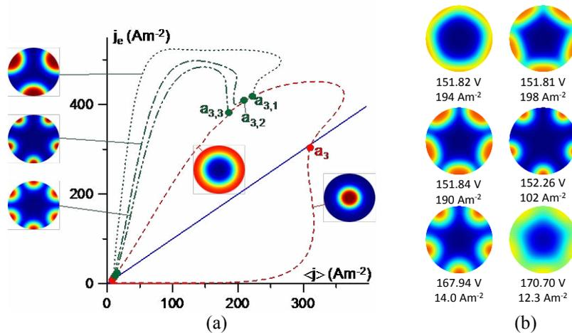
Fig. 3: Xe, 30 Torr. (a) Bifurcation diagram. Solid: the 1D mode. Dashed: 2D mode a<sub>3</sub>b<sub>3</sub>. Other lines: 3D modes. Circles: bifurcation points. b): Evolution of distribution of current on the surface of the cathode associated with the mode a<sub>3,2</sub>b<sub>3,2</sub>.
