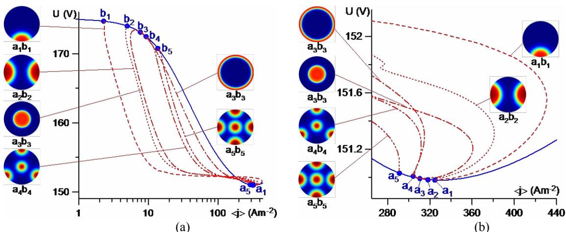
Fig. 1: CVCs. Xe, 30 Torr. Solid: the 1D mode. Dashed-dotted: 2D mode  $a_3b_3$ . Other lines: different 3D modes. Circles: bifurcation points. a): General view. b): Details near the point of minimum of the CVC of the 1D mode.
