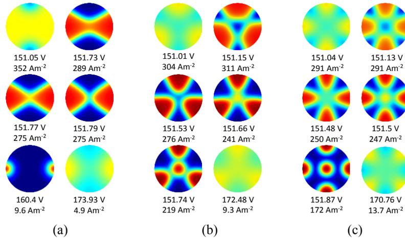
Fig. 2: Evolution of distributions of current on the surface of the cathode associated with different modes. Xe, 30 Torr. a): mode a<sub>2</sub>b<sub>2</sub>. b): a<sub>4</sub>b<sub>4</sub>. c): a<sub>5</sub>b<sub>5</sub>.
